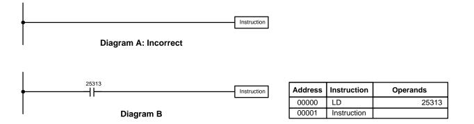
There are a few exceptions to this rule, including the INTERLOCK CLEAR, JUMP END, and step instructions. Each of these instructions is used as the second of a pair of instructions and is controlled by the execution condition of the first of the pair. Conditions should not be placed on the instruction lines leading to these instructions. Refer to *Section 5 Instruction Set* for details.
